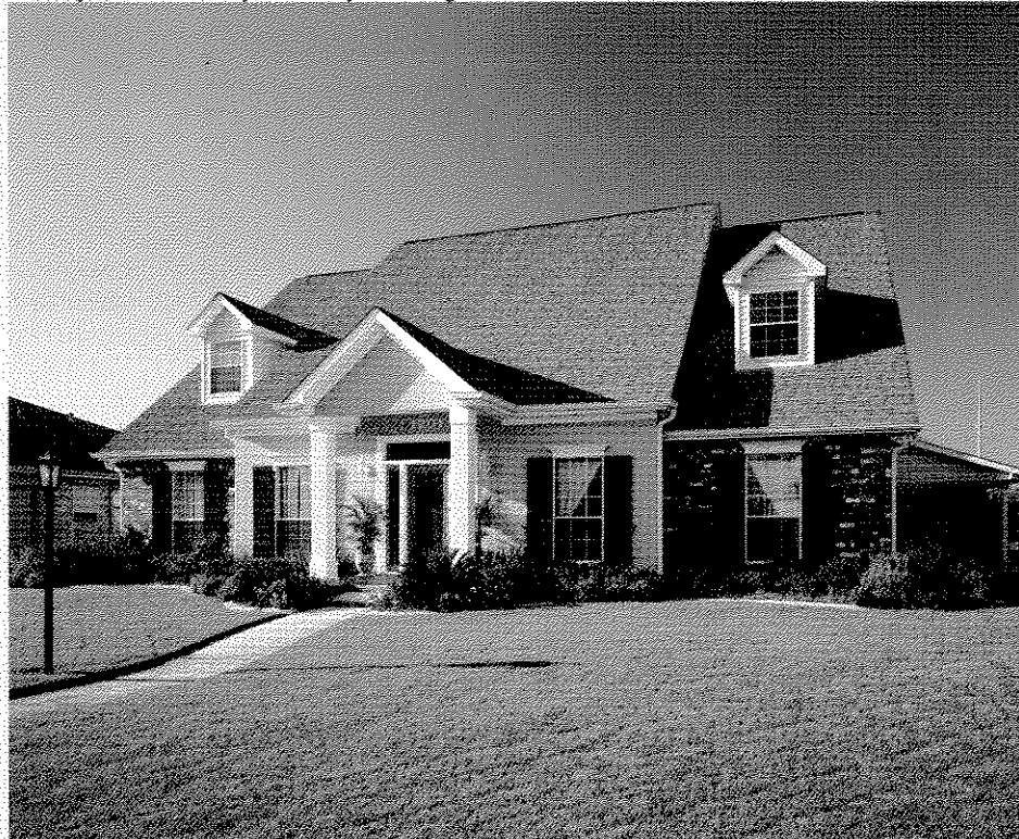
This 4,700-square-foot, contemporary Acadian home is a bonus for the neighborhood. What curb appeal! This home features a brick and stucco facade, pediments above the windows, fluted columns, leaded-glass front door and transom and sidelight, dentil block frieze board, operable wooden shutters, brick front porch, dimensional shingles and insulated windows. Brick by GATS Masonry. Photo by Joe Bergeron, M. Photo, C.P.P.
